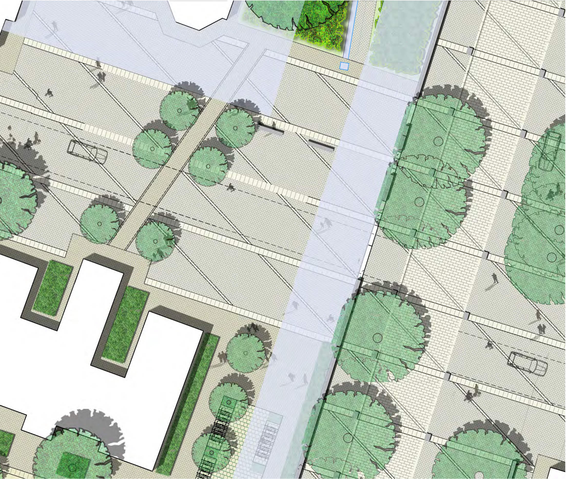
rhomboid paving with slab frame, small cobbles and large sett for traffic zone
